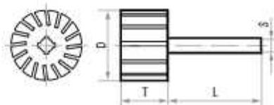
The stated maximum permissible speeds apply for a maximum overhang length  $L_0$  of 20 mm. The maximum permissible speed must be calculated separately for other overhang lengths!
