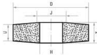
■ grinding wheel as per ISO 603-12 in SE4 shape
