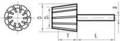
The stated maximum permissible speeds apply for a maximum overhang length  $L_0$  of 20 mm. The maximum permissible speed must be calculated separately for other overhang lengths!
