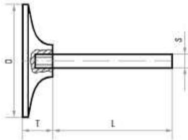
The specified maximum permissible speeds apply for a maximum overhang length  $L_0$  of 20 mm. The maximum permissible speed must be calculated separately for other overhang lengths.
